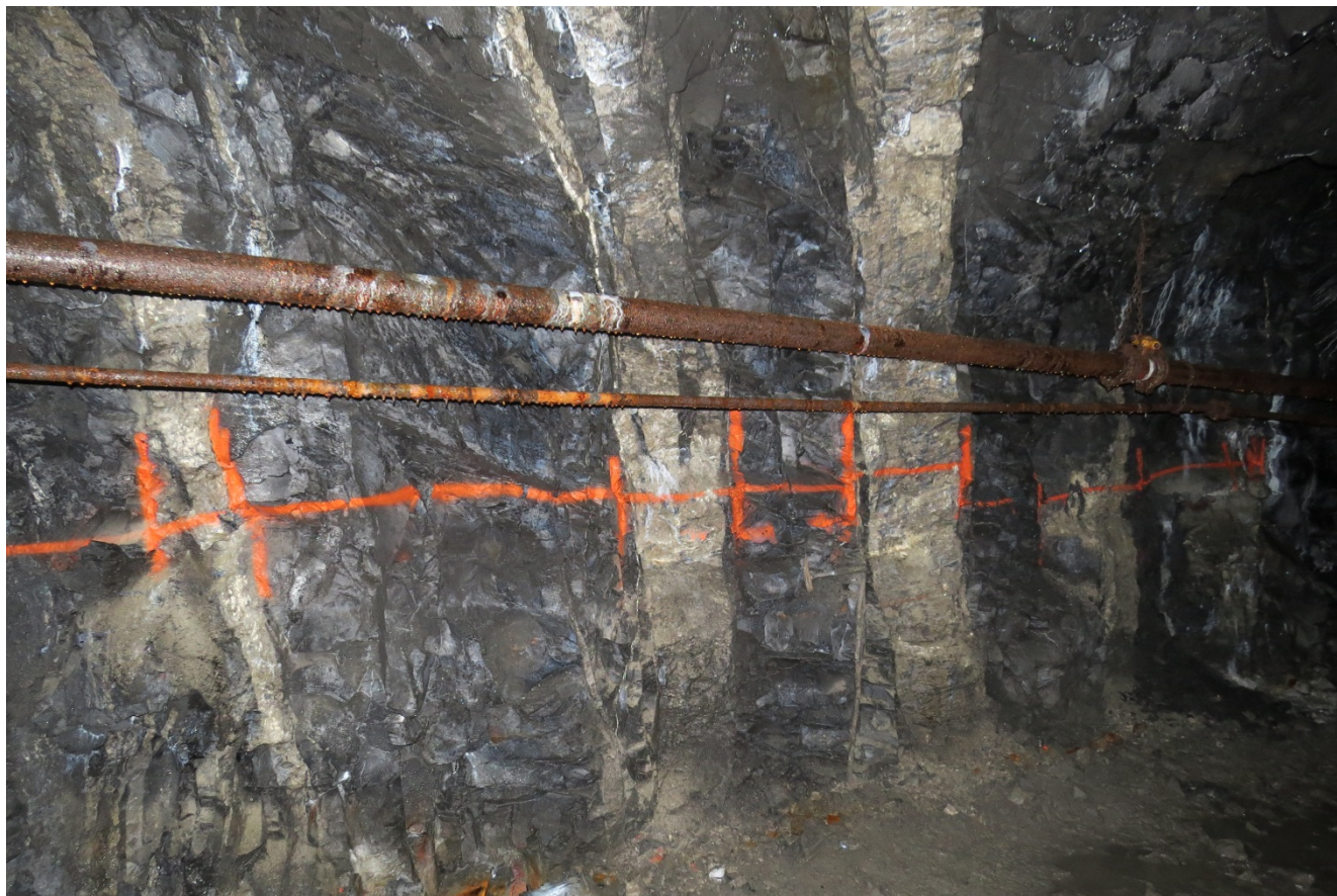
Figure 7.5 Stockwork Mineralization showing separate distinct high-grade sub-vertical veins in 880 mL
